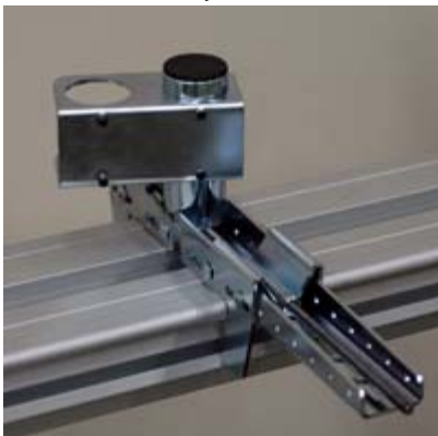
7. Turn 4 set screws into the holes in one tube yoke and slide the tube yoke onto the tube of the T-support. Rotate the yoke to approximate position and tighten down the set screws against the tube.
