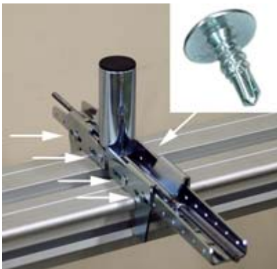
4. Place the T-support with the M-grips in position onto a work surface and drive 4 self-tap screws into the slotted holes of the M-Grips and into the round holes of the T-support on both sides. Tighten all 8 screws, then back them off half a turn. Return the assembly to the saw stand.
