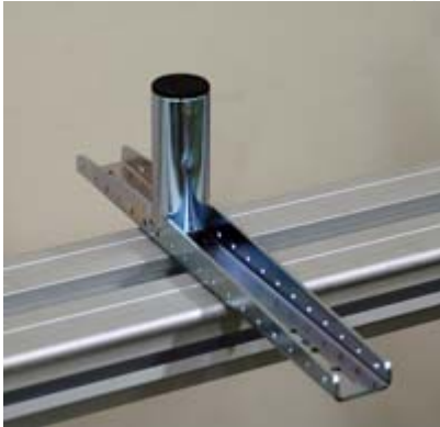
1. Place one plugged T-support on the saw stand.
